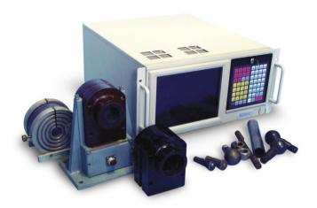
Eddy current coercimeter VS-2010 is intended for incoming inspection in implementation of continuous grading of ferrous rolled metal products: pipes, wire rods, strands and for grading according to thermal treating conditions of homogeneous parts. Presorting according to steel grade, hardness and ultimate stress limit.
